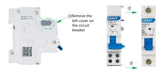
After SHT-X1 is assembled with the circuit breaker, mount them on TH35-7.5 steel mounting rail.
